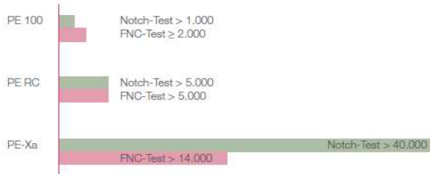
Test Results of Notch Tests & Full Notch Creep Tests (FNCT) in Hours
